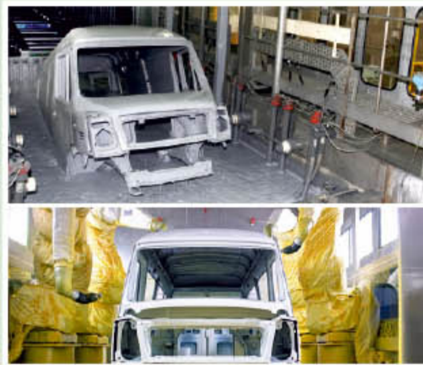
C.E.D. Primer Application and Robotic Top Coat painting for Paint Gloss Retention
