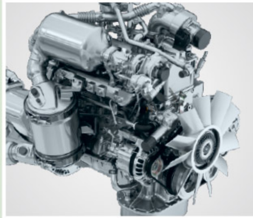
Mercedes derived, Highly Powerful and fuel efficient FM 2.6 CNG Power train
